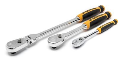
With 90 teeth, the new line of ratchets provides a 4-degree swing arc for greater access in tight spaces. The precision-engineered, high-strength pawl gives increased durability, helping the ratchets exceed ASME torque performance requirements. For those who prefer a chrome handle, the full polish versions are easy to clean and ergonomic to be easier on the hands. For those who prefer it, the solvent-resistant cushion grip is comfortable but tough enough to handle shop life.
